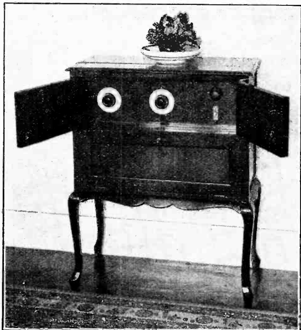
A form of cabinet in popular demand. It contains receiving set, battery eliminator and frame aerial and gives continuous service from a power point.
